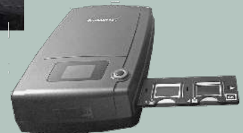
FibreShape D with a real optical resolution of 7µm. Natural fibers and recycled glass fibers with a size range of 12µm-1cm (L) / 10µm – 100µm (W) can be measured.
