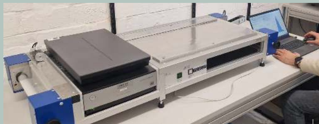
FibreShape FA with Samplefeeder Automatic for the analysis of wood shives, hemp hurd and recycled glass fibers.
